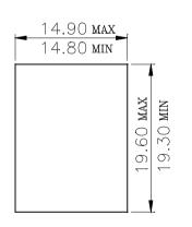
Single Panel-Latch Clearance Panel Thickness 0.062 inch.
