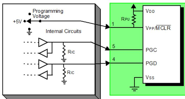
For programming, no clock is needed on the target device, but power must be supplied. When programming, the debugger puts programming levels on VPP/MCLR, sends clock pulses on PGC, and serial data via PGD. To verify that the part has been programmed correctly, clocks are sent to PGC and data is read back from PGD. This sequence confirms the debugger and device are communicating correctly.
