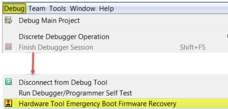
The figure below shows where the emergency recovery button is located on the MPLAB PICKit 5 In-Circuit Debugger.
