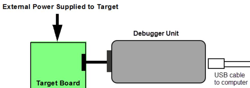
**Note:** A target powered by an external supply may power the debugger during Programmer-To-Go operation.
