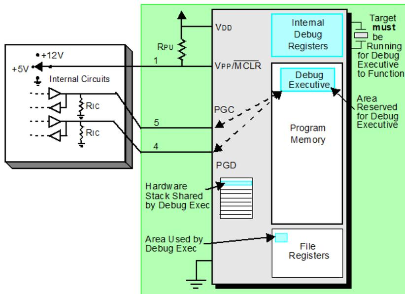
To find out whether an application program will run correctly, a breakpoint is typically set early in the program code. When a breakpoint is set from the user interface of MPLAB X IDE, the address of the breakpoint is stored in the special internal debug registers of the target device. Commands on PGC and PGD communicate directly to these registers to set the breakpoint address.
