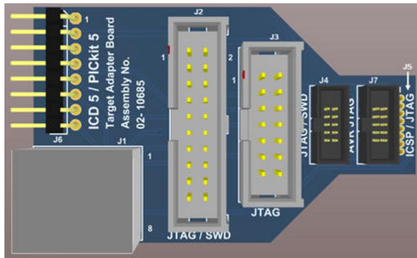
**Table 10-5.** Debugger Adapter Board - Target Connections
