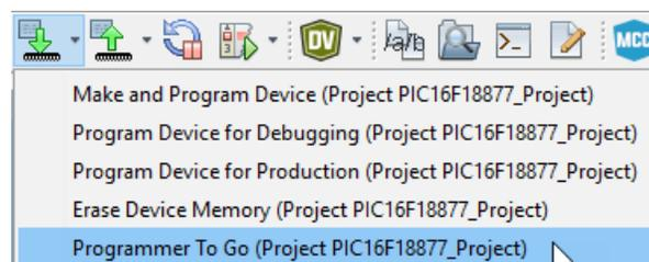
During this process, the device is programmed, then the microSDHC card is populated with the appropriate files for the Programmer-To-Go operation. The Output window displays a status message “Programming/Verify complete” when the process finishes successfully.
