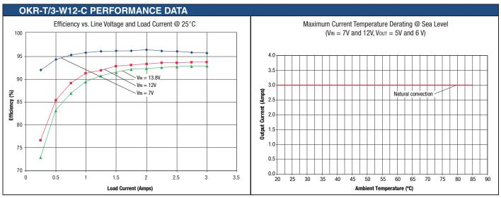
There is no derating for Vout = 0.591V. to 5.5V. at full load.
