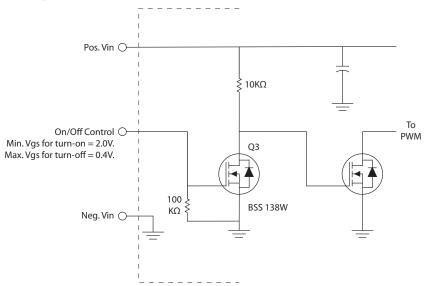
Figure 6. On/Off Control Circuit for "E" Models
