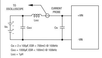
Figure 4. Measuring Input Ripple Current
