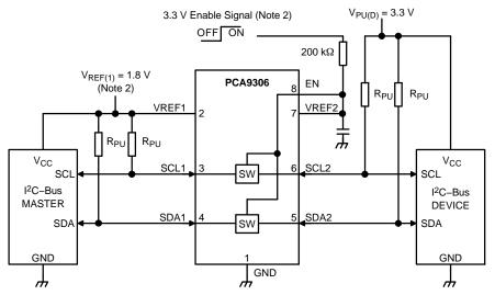
2. In the Enabled mode, the applied enable voltage and the applied voltage at  $V_{ref(1)}$  should be such that  $V_{bias(ref)(2)}$  is at least 1 V higher than  $V_{ref(1)}$  for best translator operation.
