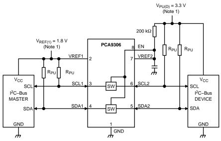
The applied voltages at V<sub>ref(1)</sub> and V<sub>pu(D)</sub> should be such that V<sub>bias(ref)(2)</sub> is at least 1 V higher than V<sub>ref(1)</sub> for best translator operation.
