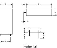
Part Numbering System Ρ HB 5 R 0 \_ R Series Voltage (V) Capacitance (µF) RoHS Code Version R = Decimal Configuration Value Multiplier V = Vertical Compliant P = Pack5R0 = 5.0VExample: 155 = 15 x 10<sup>5</sup>µF or 1.5F H = Horizontal
