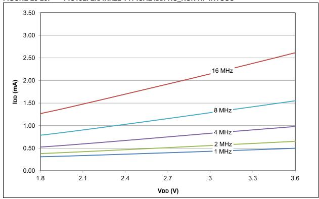
FIGURE 28-27: PIC18LF2X/4XK22 MAXIMUM IDD: RC\_RUN HF-INTOSC
