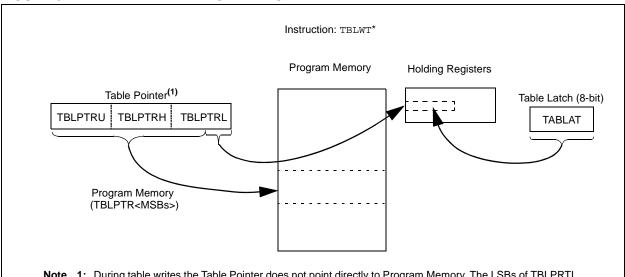
Note 1: During table writes the Table Pointer does not point directly to Program Memory. The LSBs of TBLPRTL actually point to an address within the write block holding registers. The MSBs of the Table Pointer determine where the write block will eventually be written. The process for writing the holding registers to the program memory array is discussed in Section 6.6 "Writing to Flash Program Memory".
