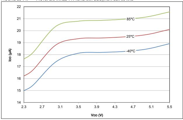
FIGURE 28-75: PIC18F2X/4XK22 MAXIMUM IDD: SEC\_RUN 32.768 kHz
