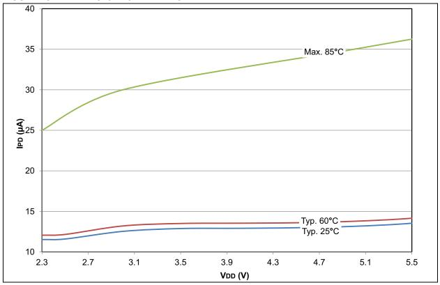
FIGURE 28-3: PIC18LF2X/4XK22 DELTA IPD WATCHDOG TIMER (WDT)
