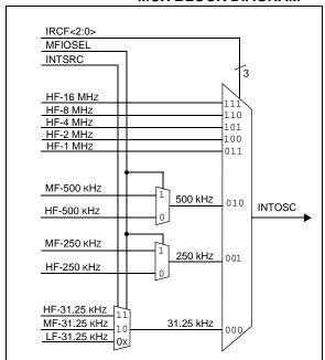
FIGURE 2-3: PLL\_SELECT BLOCK DIAGRAM
