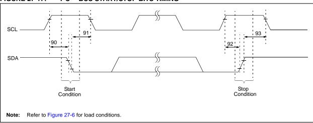
TABLE 27-16: I<sup>2</sup>C™ BUS START/STOP BITS REQUIREMENTS (SLAVE MODE)
