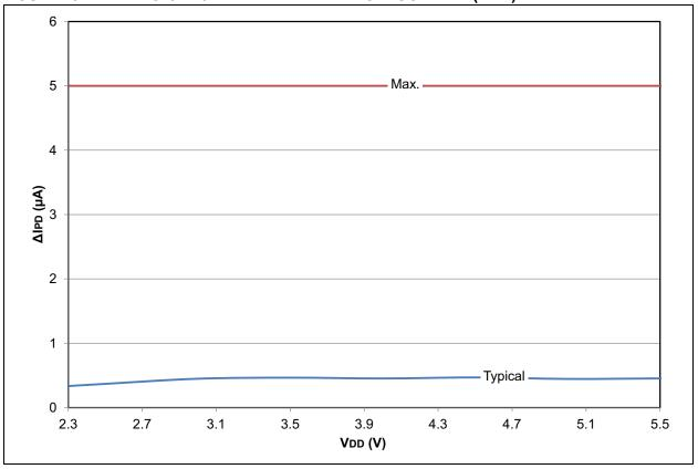
FIGURE 28-5: PIC18LF2X/4XK22 DELTA IPD BROWN-OUT RESET (BOR)
