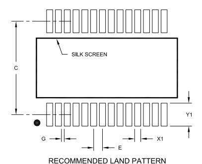
Units **MILLIMETERS Dimension Limits** MIN NOM MAX Contact Pitch 0.65 BSC Ε Contact Pad Spacing С 7.20 Contact Pad Width (X28) X1 0.45 Contact Pad Length (X28) Y1 1.75 Distance Between Pads G 0.20
