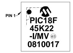
44-Lead QFN (8x8x0.9 mm)
