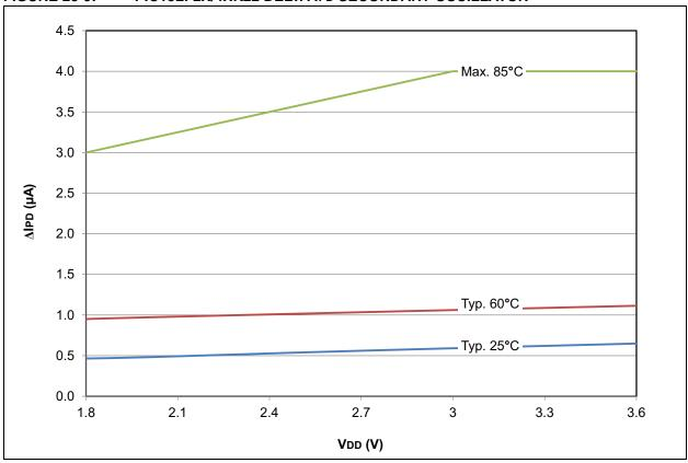
FIGURE 28-10: PIC18F2X/4XK22 DELTA IPD SECONDARY OSCILLATOR
