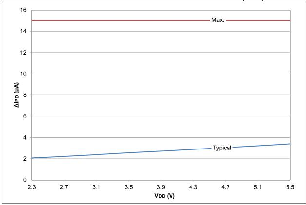
FIGURE 28-9: PIC18LF2X/4XK22 DELTA IPD SECONDARY OSCILLATOR
