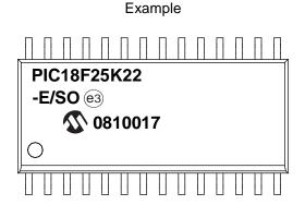
28-Lead SSOP (5.30 mm)
