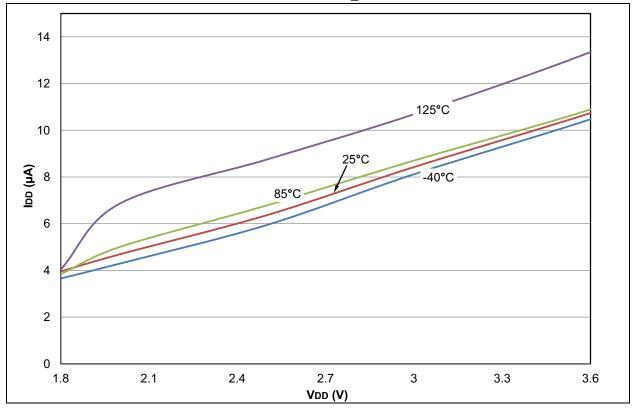
FIGURE 28-21: PIC18LF2X/4XK22 MAXIMUM IDD: RC\_RUN LF-INTOSC 31 kHz
