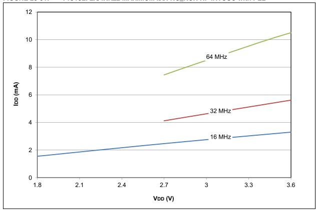
FIGURE 28-32: PIC18F2X/4XK22 TYPICAL IDD: RC\_RUN HF-INTOSC with PLL
