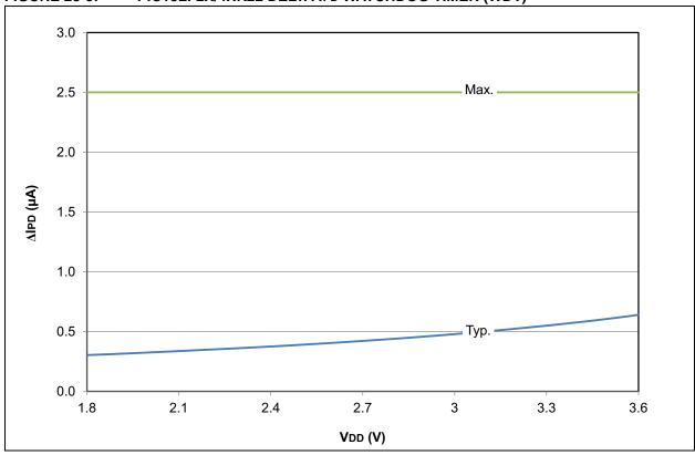
FIGURE 28-4: PIC18F2X/4XK22 DELTA IPD WATCHDOG TIMER (WDT)
