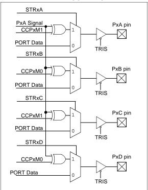
Note 1: Port outputs are configured as shown when the CCPxCON register bits PxM<1:0> = 00 and CCPxM<3:2> = 11.
