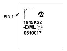
44-Lead TQFP (10x10x1 mm)
