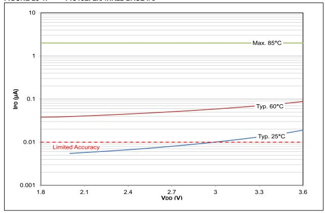
FIGURE 28-2: PIC18F2X/4XK22 BASE IPD
