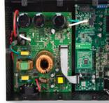
This development system is intended for high-voltage (up to 400 volts at 6.5 amps) BLDC, PMSM and ACIM sensored or sensorless applications. It provides a low-cost Integrated Power Module (IPM) based system for users
