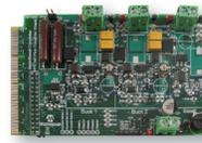
A low-cost development platform for dsPIC33F ‘GS’ devices, the buck/boost converter PICTail Plus card has two buck stage outputs and one boost stage output. Various performance measures
