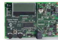
This starter kit allows the user to easily explore the capabilities and features of the dsPIC33F GS Digital Power Conversion family. It is a digitally controlled power supply board that
