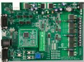
This development board is intended for low-voltage (up to 48 volts at 10 amps) BLDC sensored or sensorless applications. It provides a low-cost system for users to evaluate and
