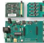
This LED lighting development kit enables designers to quickly leverage the capabilities and performance of the dsPIC33 ‘GS’ DSCs to create a 100% digitally controlled ballast function, while including advanced features such as
