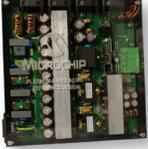
This reference design demonstrates the flexibility and power of dsPIC Digital Signal Controllers in Switch Mode Power Supplies. This reference design has a peak efficiency of 94.1% and achieves the ENERGY STAR® CSCI Platinum Level. It features a 2-phase
