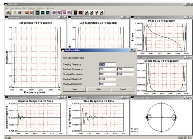
The Digital Filter Design Tool makes designing and analyzing FIR and IIR filters easy. When the user enters frequency specifications, the tool automatically generates the filter code and coefficients. Graphical output windows provide the desired filter's characteristics.
