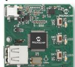
These starter kits provide a low-cost modular development system for Microchip's enhanced 16-bit DSCs or high-performance MCUs. They come with preloaded demo software to allow the user to explore the new features of the dsPIC33E DSC family or the PIC24E MCU family.
