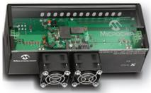
This reference design provides an easy method to evaluate the performance and features of SMPS DSCs in high-density quarter brick DC-DC converters for Intermediate Bus Architectures
