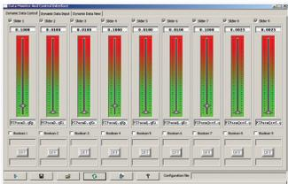
The Real-Time Data Monitor saves development and testing time for embedded control applications. RTDM allows users to make a change to a software parameter and see the effect immediately without
