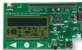
This kit includes an analog header for clean analog signals and plugs into breadboards. The board includes connections for microphone, headphones as well as on-board light and temperature sensors. The
