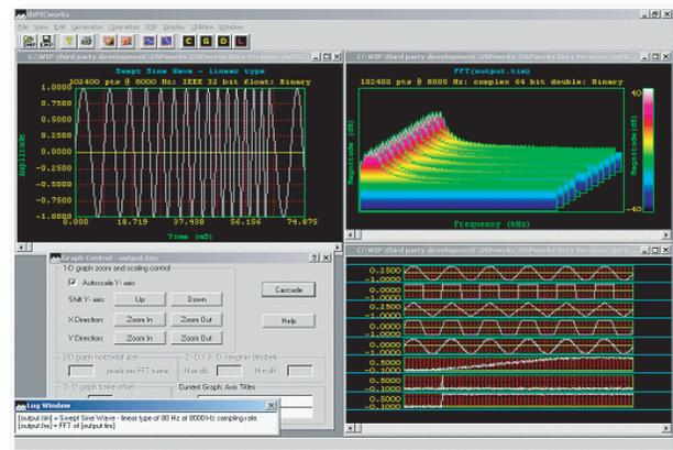
The dsPICworks Data Analysis and DSP Software makes it easy to evaluate and analyze DSP algorithms. You can run a variety of DSP and arithmetic operations and analyze your data in both time and frequency domain.
