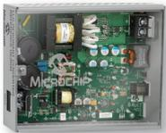
This reference design operates over a wide input voltage range (350-420V DC) with a nominal input of 400V, providing a 12V DC output while maintaining high-voltage isolation between the primary and secondary. This reference
