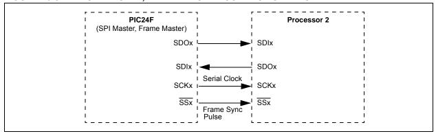
FIGURE 16-6: SPI MASTER, FRAME SLAVE CONNECTION DIAGRAM
