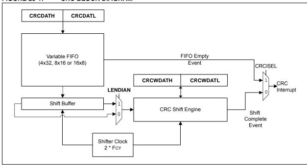
FIGURE 23-2: CRC SHIFT ENGINE DETAIL
