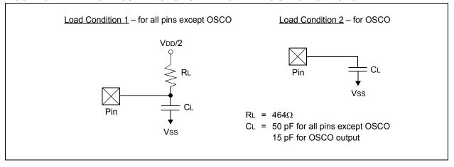
**TABLE 32-18: CAPACITIVE LOADING REQUIREMENTS ON OUTPUT PINS**
