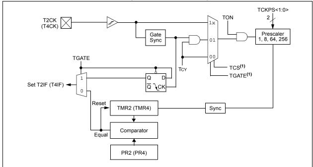
Note 1: The timer clock input must be assigned to an available RPn/RPIn pin before use. See Section 11.4 "Peripheral Pin Select (PPS)" for more information.
