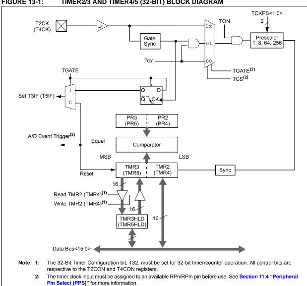
The A/D event trigger is available only on Timer 2/3 in 32-bit mode and Timer 3 in 16-bit mode.
