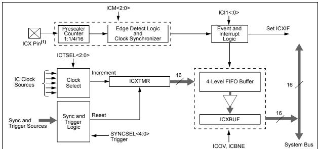
Note 1: The ICx inputs must be assigned to an available RPn/RPIn pin before use. See Section 11.4 "Peripheral Pin Select (PPS)" for more information.
