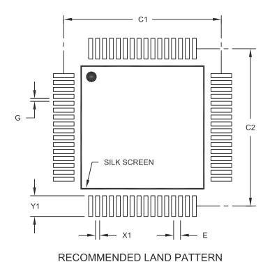
MILLIMETERS Units **Dimension Limits** MIN NOM MAX 0.50 BSC Contact Pitch Ε Contact Pad Spacing C1 11.40 Contact Pad Spacing C2 11.40 Contact Pad Width (X64) X1 0.30 Contact Pad Length (X64) Y1 1.50 0.20 Distance Between Pads G
