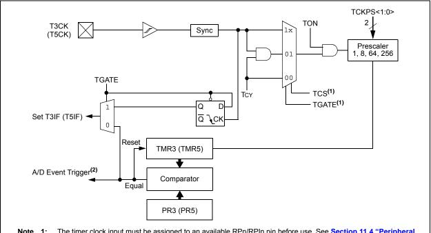
Note 1: The timer clock input must be assigned to an available RPn/RPIn pin before use. See Section 11.4 "Peripheral Pin Select (PPS)" for more information.
