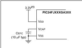
Note 1: This is a typical operating voltage. Refer to Section 32.0 "Electrical Characteristics" for the full operating ranges of VDD.
