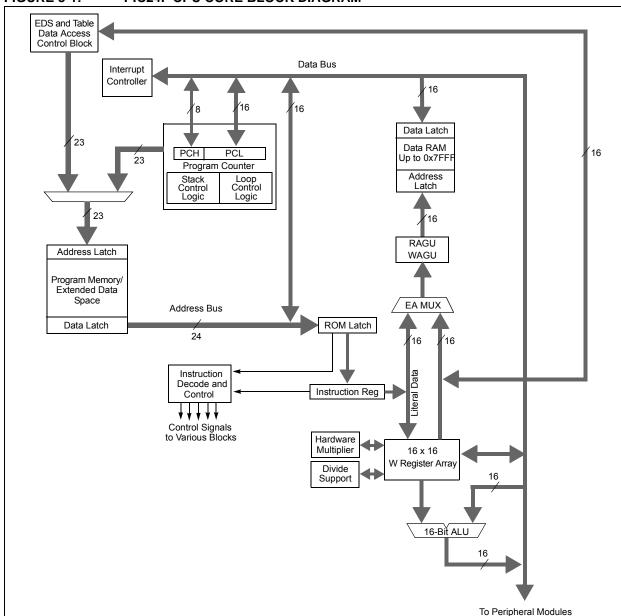
FIGURE 3-1: PIC24F CPU CORE BLOCK DIAGRAM
