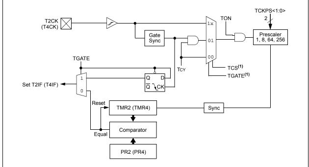
Note 1: The timer clock input must be assigned to an available RPn pin before use. Please see Section 10.4 "Peripheral Pin Select (PPS)" for more information.
