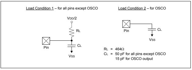
**TABLE 29-15: CAPACITIVE LOADING REQUIREMENTS ON OUTPUT PINS**
