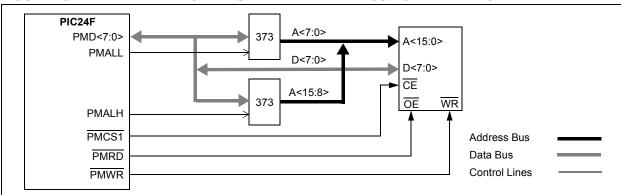
FIGURE 19-8: EXAMPLE OF A PARTIALLY MULTIPLEXED ADDRESSING APPLICATION
