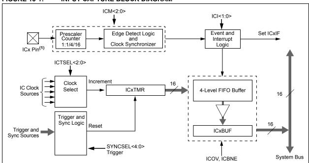
Note 1: The ICx inputs must be assigned to an available RPn pin before use. Please see Section 10.4 "Peripheral Pin Select (PPS)" for more information.
