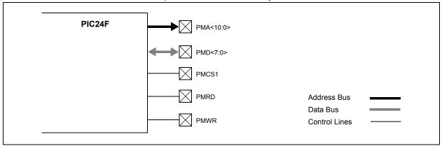
FIGURE 19-5: MASTER MODE, PARTIALLY MULTIPLEXED ADDRESSING (SEPARATE READ AND WRITE STROBES, SINGLE CHIP SELECT)
