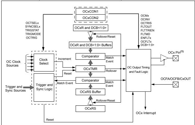
Note 1: The OCx outputs must be assigned to an available RPn pin before use. Please see Section 10.4 "Peripheral Pin Select (PPS)" for more information.
