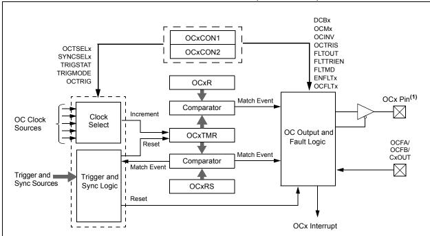
Note 1: The OCx outputs must be assigned to an available RPn pin before use. Please see Section 10.4 "Peripheral Pin Select (PPS)" for more information.
