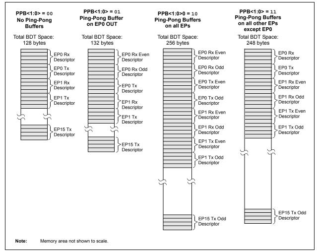
BDs have a fixed relationship to a particular endpoint, depending on the buffering configuration. Table 18-2 provides the mapping of BDs to endpoints. This relationship also means that gaps may occur in the BDT if endpoints are not enabled contiguously. This theoretically means that the BDs for disabled endpoints could be used as buffer space. In practice, users should avoid using such spaces in the BDT unless a method of validating BD addresses is implemented.
