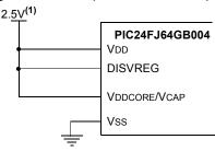
Note 1: These are typical operating voltages. Refer to Section 29.1 "DC Characteristics" for the full operating ranges of VDD and VDDCORE.
