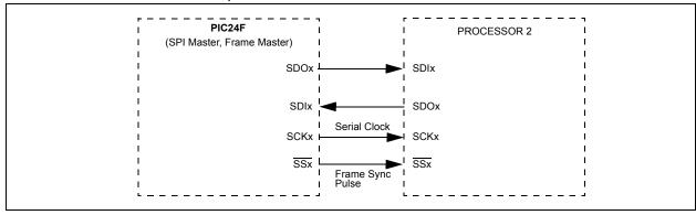
FIGURE 15-6: SPI MASTER, FRAME SLAVE CONNECTION DIAGRAM
