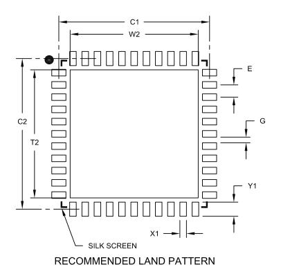
Units **MILLIMETERS** MIN MOM MAX **Dimension Limits** Contact Pitch Е 0.65 BSC Optional Center Pad Width W2 6.80 Optional Center Pad Length T2 6.80 Contact Pad Spacing C1 8.00 Contact Pad Spacing C2 8.00 Contact Pad Width (X44) X1 0.35 Contact Pad Length (X44) <u>Y1</u> 0.80 G 0.25 Distance Between Pads
