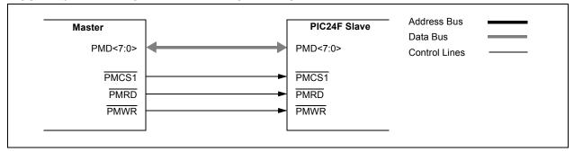
FIGURE 19-3: ADDRESSABLE PARALLEL SLAVE PORT EXAMPLE
