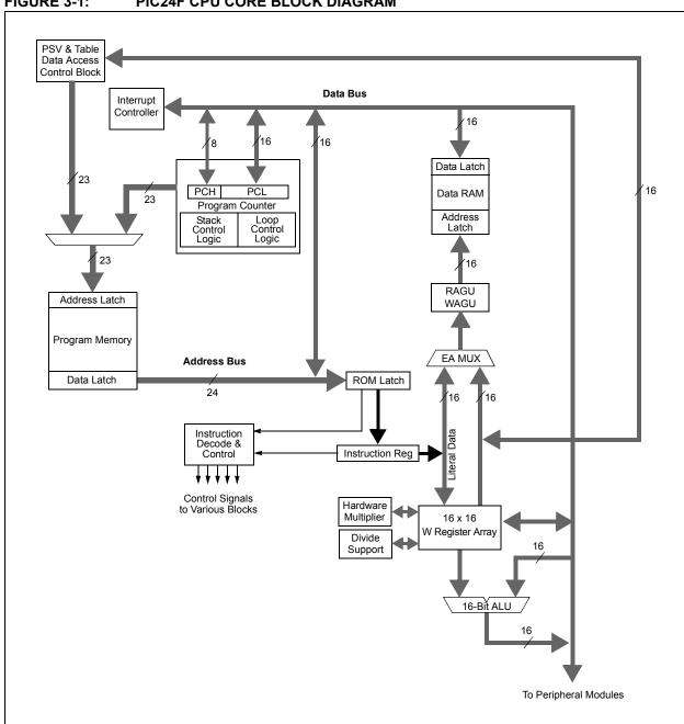
FIGURE 3-1: PIC24F CPU CORE BLOCK DIAGRAM
