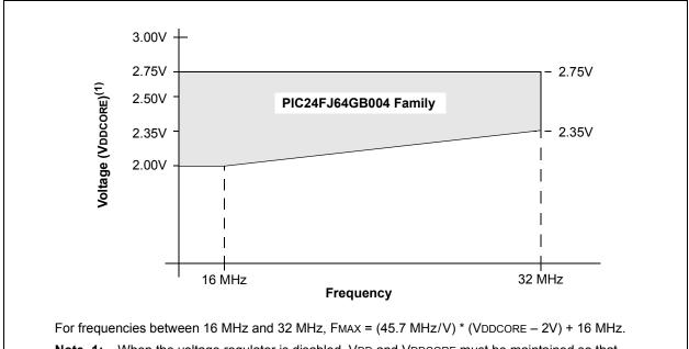
Note 1: When the voltage regulator is disabled, VDD and VDDCORE must be maintained so that  $VDDCORE \le VDD \le 3.6V$ .
