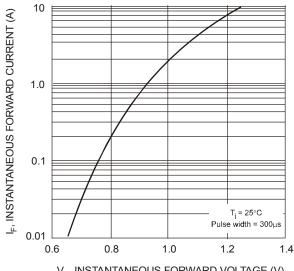
$V_{\text{F}}$ , INSTANTANEOUS FORWARD VOLTAGE (V) Fig. 2 Typical Forward Characteristics
