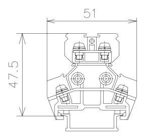
The CTW terminal blocks of a compact design (terminal pitch: 8mm) can have the required terminal block space inside your panels. These terminal blocks are suited for use in operation panels, control panels and instrumentation panels, especially for use in sequencer mounting panels.
