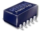
Both converters are available in SMD mount packages as the R-78Axx-0.5SMD or the R-78Axx-1.0SMD. The extra pins offered by the SMD package allows two additional functions to be built into these versions: remote On/Off control and output voltage trim. The output voltage can be adjusted over a range of about +/- 50% using a single external resistor and the remote on/off control puts the converters into ultra-low power mode where they draw only 20  $\mu$ A current!
