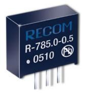
The R-78xx-0.5 offers output voltages from 1.5V to 15VDC at a maximum output current of 0.5A with the full input voltage range of up to 34VDC. The SIP3 package measures only  $11.5 \times 10 \times 8$ mm (0.45 x 0.4 x 0.3"), yet delivers up to 7.5 Watts of power. The R-78xx-1.0 offers output voltages from 1.8V to 5VDC at a maximum output current of 1A with a reduced input voltage range of 4.75 to 18VDC in the same package.
