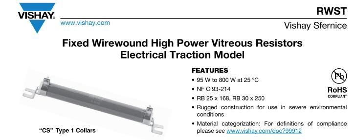
The RWST vitreous wirewound high power resistors are known for their excellent reliability which has developed out of the Vishay Sfernice experience over several decades in the field of high current applications.
