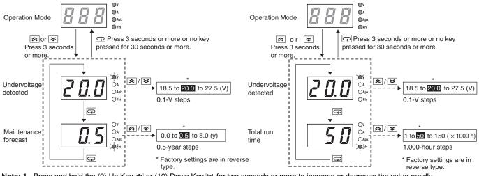
Note: 1. Press and hold the (9) Up Key 🗟 or (10) Down Key 🗹 for two seconds or more to increase or decrease the value rapidly. 2. The S8VS-06024 is not provided with the setting mode and its parameters are fixed at the shipment setting.
