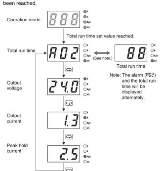
The accumulated value of the operating time of the Power Supply is displayed as the total run time.  $\square$  (kh) will be displayed initially after purchase and then the display will advance in *1*-kh steps as the operating time accumulates. When the total run time reaches the alarm set value, the alarm (RD2) and the total run time will be displayed alternately and a transistor (total run time output terminal (kh)) will output the status externally.
