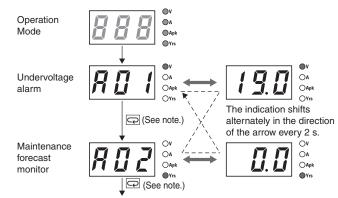
\* When undervoltage alarm is indicated: Press  $\ensuremath{\fbox{\sc constraint}}$  Key  $\rightarrow$  output load indication
