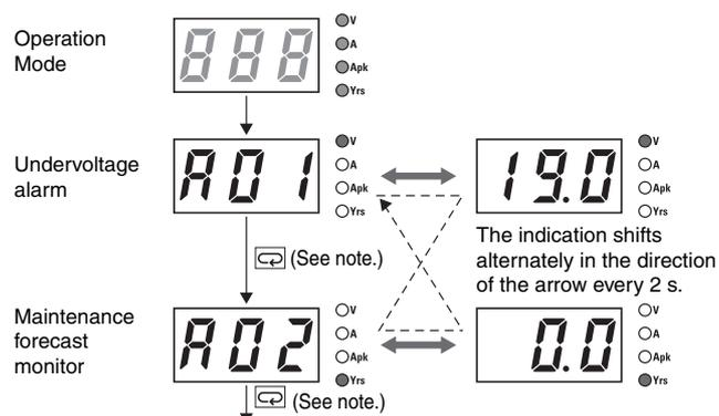
\* When undervoltage alarm is indicated: Press Key → output load indication
