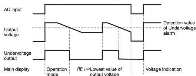
**Note:** Operation begins after about three seconds since the AC power is supplied.
