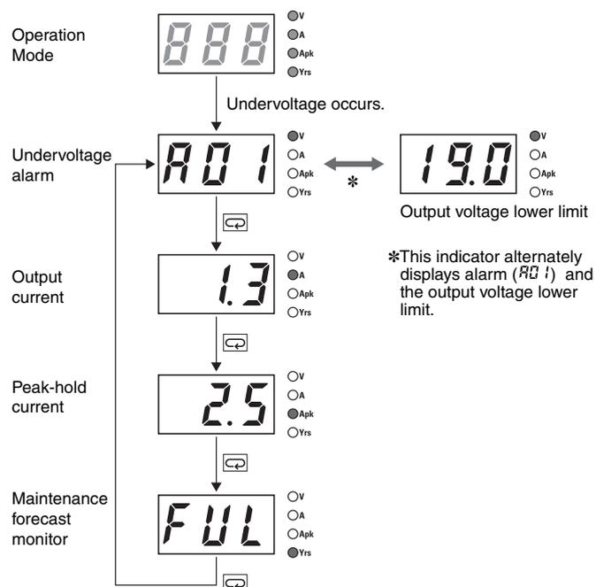
**Note: 1.** When the voltage is restored to the set value or higher and the Key is pressed at the *R01* display to return to the output current display, the *R01* alarm will be cleared and the normal output display will return.
