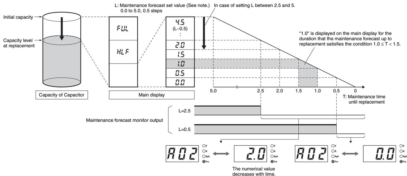
**Note:** This function can be set only on the S8VS-09024A□□, S8VS-12024A□, S8VS-18024A□, S8VS-24024A□, and S8VS-48024A.
