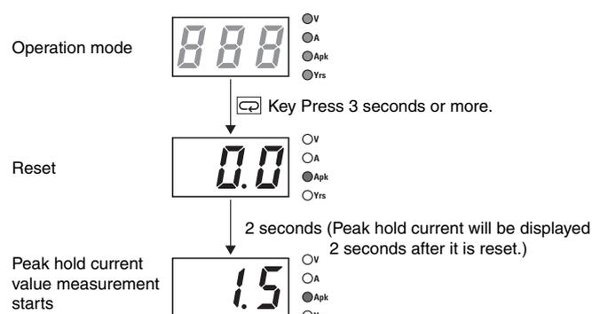
**Note:** The peak hold current value is not reset in the setting mode.
