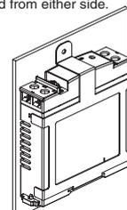
Note: The Side-mounting Bracket (S82Y-VS30P) can be mounted from either side.
