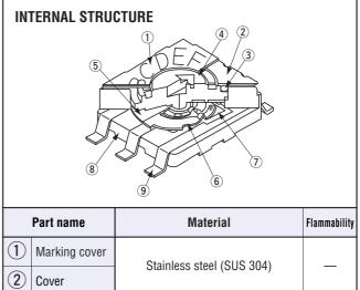
(3) "0" ring Silicone rubber UL-94HB **(4)** UL-94V-0 Rotor PPS (Polyphenylenesulphide) **(5)** Spacer Stainless steel (SUS 304) **(6)** Moving contact Copper alloy, Gold-plated Fixed contact (8) Housing UL-94V-0 PPS (Polyphenylenesulphide) **9** Terminal pin Copper alloy, Gold-plated
