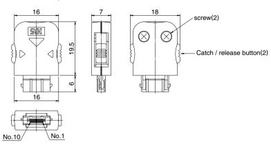
• 10 pos. (Reverse, non-shielded type, for 4mm max. cable diameter)
