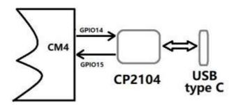
The design of console used a USB- UART converter, most OS of the computer have the driver, if not, the link below may be useful:
