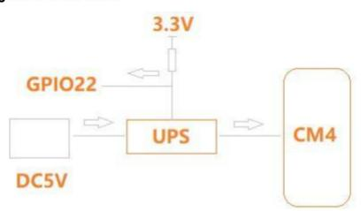
The UPS module is inserted between the DC5V and CM4, a GPIO is used to alarm CPU when the 5V power supply is down. Then the CPU should do something urgent in a script before energy exhaustion of super capacitor and run a "\$shutdown"
