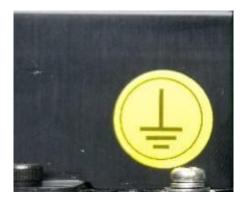
The PE signal is optional. If there is no EMI present ,the PE connection can left open.
