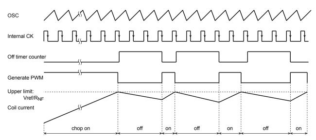
The upper limit of the current across the motor coil (i.e., the peak current in each excitation mode), I (Limit), can be calculated as follows:
