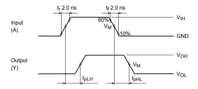
Figure 2 t<sub>pLH</sub>, t<sub>pHL</sub>
