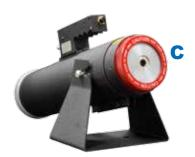
Bench mount pneumatic crimp tool. Heavy duty, four-indent crimp termination. Attach to air supply with quick-disconnect fitting or install 1/4 NPT fitting into tapped port. 90-120 psi air supply. Requires die assemblies and locators, sold separately. Hand actuate with push-button valve trigger on handle. Steel with black wrinkle enamel coating. 13 inches overall length, 9.2 inches tall, 17 pounds (7.7 Kg).
