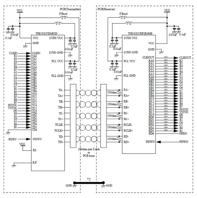
Figure 10. Typical Connection Diagram
