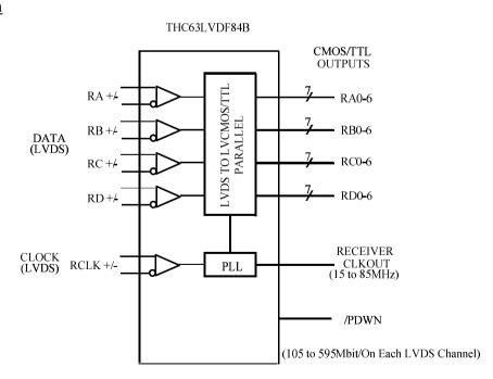
Figure 1. Block Diagram
