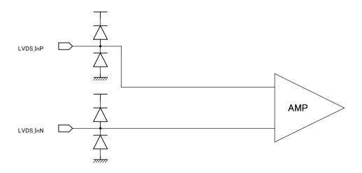
Figure 3. LVDS Input Schematic Diagram
