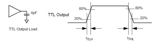
Figure 6. CLKOUT Transmission Time
