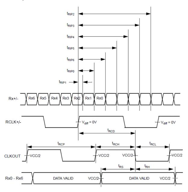
Figure 7. LVDS Input Data Position
