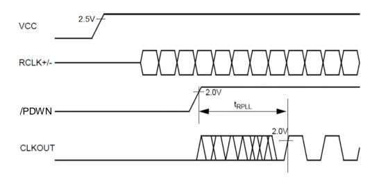
Figure 8. PLL Lock Loop Set Time
