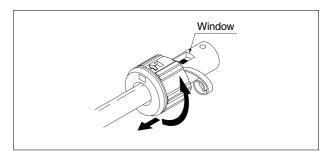
Even double layer polyurethane tubing (series TRBU) which is highly adhesive to the external layer can be stripped easily.
