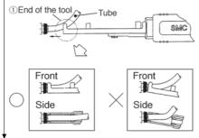
After inserting, grasp the handle tightly and insert the end of the tubing to the stroke end.
