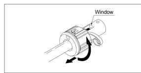
• Even double layer polyurethane tubing (series TRBU) which is highly adhesive to the external layer can be stripped easily.
