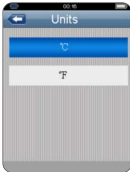
Press the UP and DOWN button to select the units, press the ESC button to esc and save.
