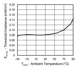
Fig. 9 - Sensitivity vs. Ambient Temperature
