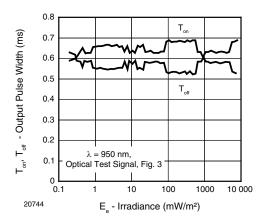
Fig. 4 - Output Pulse Diagram
