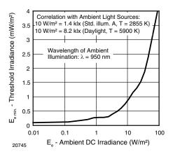
Fig. 6 - Sensitivity in Bright Ambient
