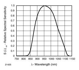
Fig. 10 - Relative Spectral Sensitivity vs. Wavelength
