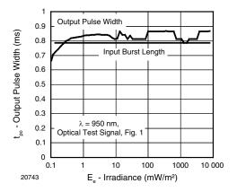
Fig. 2 - Pulse Length and Sensitivity in Dark Ambient
