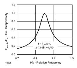
Fig. 5 - Frequency Dependence of Responsivity
