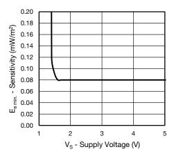
Fig. 12 - Sensitivity vs. Supply Voltage
