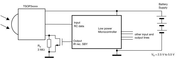
Fig. 9 - Circuit Proposal for Pulsing the Supply Voltage of the TSOP3xxxx
