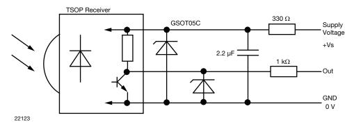
Fig. 2 - Protection Circuit against Over Voltage Spikes
