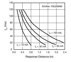
Fig. 7 - t<sub>po</sub> vs. Distance Kodak Gray Card Plus 15 %
