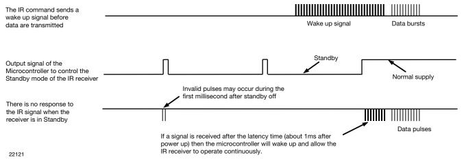
Fig. 8 - Example for a Battery-Saving Mode with TSOP3xxxx IR Receivers
