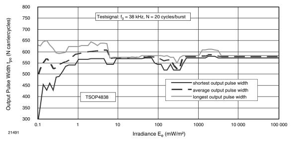
Fig. 1 - Statistical Evaluation of 1000 Output Pulses at each Irradiance
