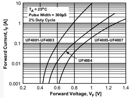
Figure 2. Forward Characteristics
