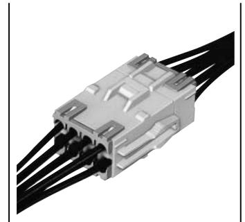
The VL connector is a 6.2mm (.244") pitch wire-to-wire connector designed for circuits requiring up to 20A (1 or 2-circuit with AWG #12 wire).
