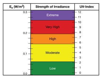
Fig. 6 - Strength of Irradiance and the UV-Index
