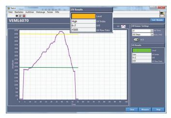
Fig. 15 - View of the VEML6070 Demo Software Showing Raw Data, UVI, and Risk Level
