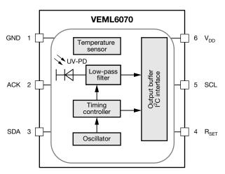
Fig. 1 - Block Diagram of the VEML6070
