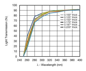
Fig. 8 - Light Transmission of ACRYLITE OP-4 Sheet (www.aetnaplastics.com/site\_media/media/documents/Acrylite\_OP-4 Material\_Data\_Sheet.pdf)
