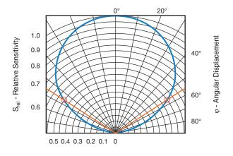
Fig. 9 - Relative Radiant Sensitivity vs. Angular Displacement
