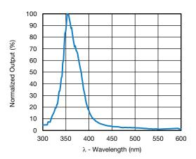
Fig. 3 - Relative Responsivity vs. Wavelength
