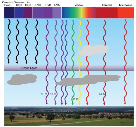
Fig. 5 - Radiation that Reaches the Earth's Surface
