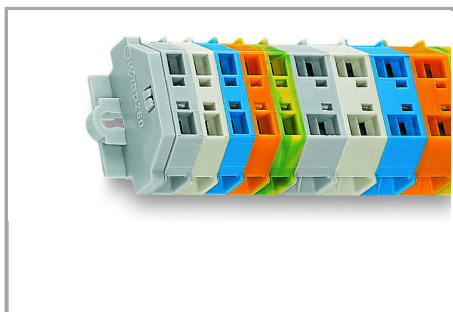
Terminal strip, with mounting flanges, for screw or similar mounting types, 3.2 mm mounting hole diameter (with 209-123 Mounting Foot for DIN-35 rail)
