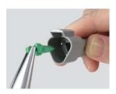
**Step 1:**Remove green wedge using needlenose pliers to pull wedge straight out.
