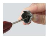
**Step 2:** To remove the contacts, gently pull wire backwards, while at the same time releasing the locking finger by moving it away from the contact with a screwdriver.
