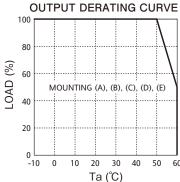
Recommended minimum air velocity: 0.7m/s (Measured at component side of PCB, air must flow through component side.)
