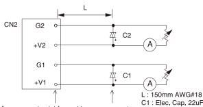
Measurement point for Measurement point Vo Line/Load Regulation for Vripple
