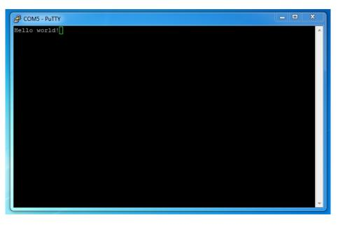
If you don't see anything, make sure you've connected the D0 pin to the D1 pin on the FT232H board.
