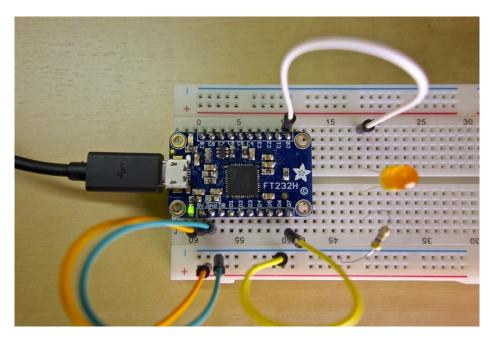
With this configuration pin **CO** will be a digital output that controls if the LED is on or off, depending on the level of the **CO** output. Pin **D7** will be a digital input that reads if it's at a high level (3-5 volts) or low level (ground).
