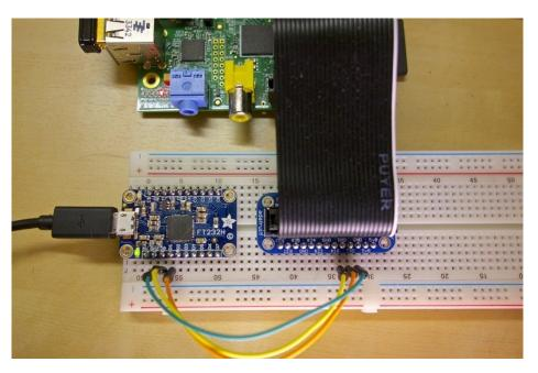
Use PuTTY or screen to open the FT232H serial port at 115200 baud and you'll be accessing the Raspberry Pi's serial port!
