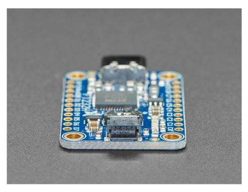
NEW: As of Feb 12, 2020 we have given this venerable board a makeover! We now have a modern USB C connector on the board (instead of micro USB), a I2C switch to connect D1 and D2 for easy I2C interfacing, 3V power output pin
