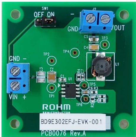
Figure 1. BD9E302EFJ-EVK-001 (Top View)
