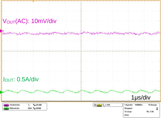
Figure 23. V_{out} Ripple ( V_{CC}=12V , I_{out}=50mA , V_{out}=3.3V )
