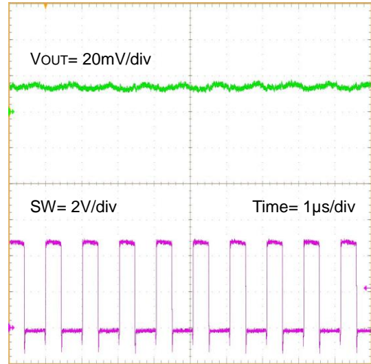
Figure 31. 出力リップル波形 ( V_{IN} = 5V , V_{OUT} = 1.8V , I_{OUT} = 3A )
