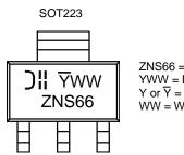
$\begin{array}{l} \text{ZNS66} = \text{Product Type Marking Code} \\ \text{YWW} = \text{Date Code Marking} \\ \text{Y or } \overline{\text{Y}} = \text{Last Digit of Year (ex: } 2 = 2022) \\ \text{WW} = \text{Week Code 01 to 52} \\ \end{array}$
