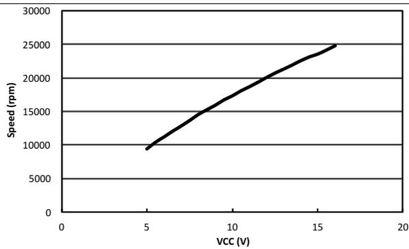
Figure 9. Fast Motor RPM vs Voltage, FS = 1
