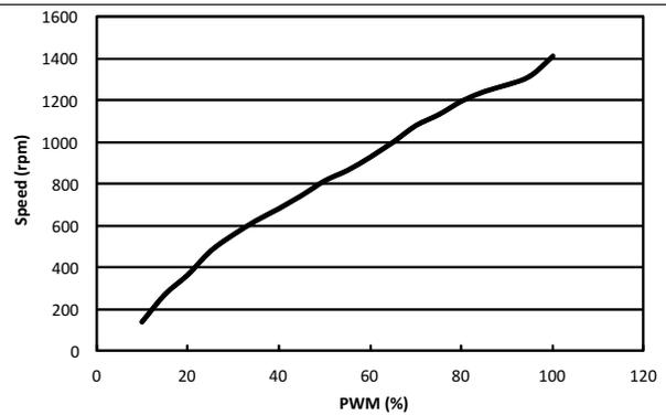
Figure 8. Slow Motor RPM vs Duty, FS = 0
