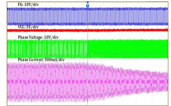
Input voltage = 12 V      PWM duty switch from 100% to 20%
