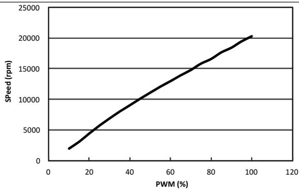
Figure 7. Fast Motor RPM vs Duty, FS = 1
