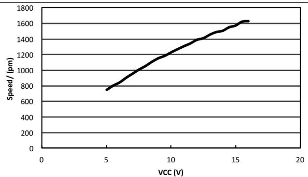
Figure 10. Slow Motor RPM vs Voltage, FS = 0
