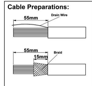
1. Prepare the cable as shown in Fig. 4 and assemble the connector
