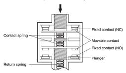
Conforms to EN60947-5-1 Direct Opening Operation ⊕
