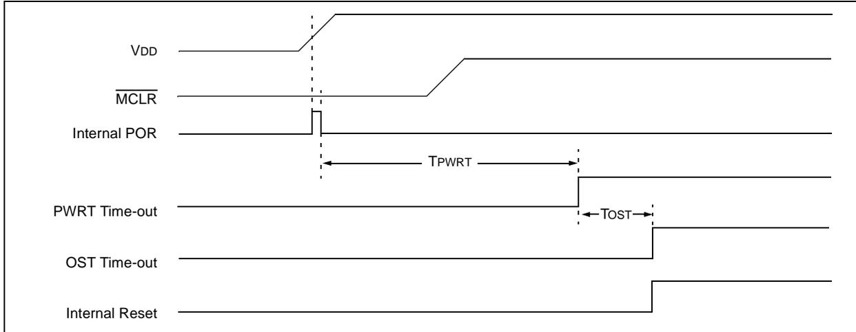
**FIGURE 12-5: TIME-OUT SEQUENCE ON POWER-UP (DELAYED  $\overline{\text{MCLR}}$ )**
