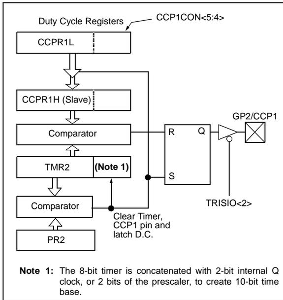
A PWM output (Figure 11-4) has a time base (period) and a time that the output stays high (duty cycle). The frequency of the PWM is the inverse of the period (1/period).
