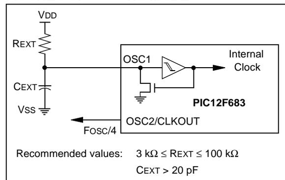
In RCIO mode, the RC circuit is connected to the OSC1 pin. The OSC2 pin becomes an additional general purpose I/O pin. The I/O pin becomes bit 4 of GPIO (GP4). Figure 3-6 shows the RCIO mode connections.
