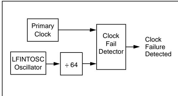
The FSCM function is enabled by setting the FCMEN bit in the Configuration Word register (CONFIG). It is applicable to all external clock options (LP, XT, HS, EC, RC or IO modes).
