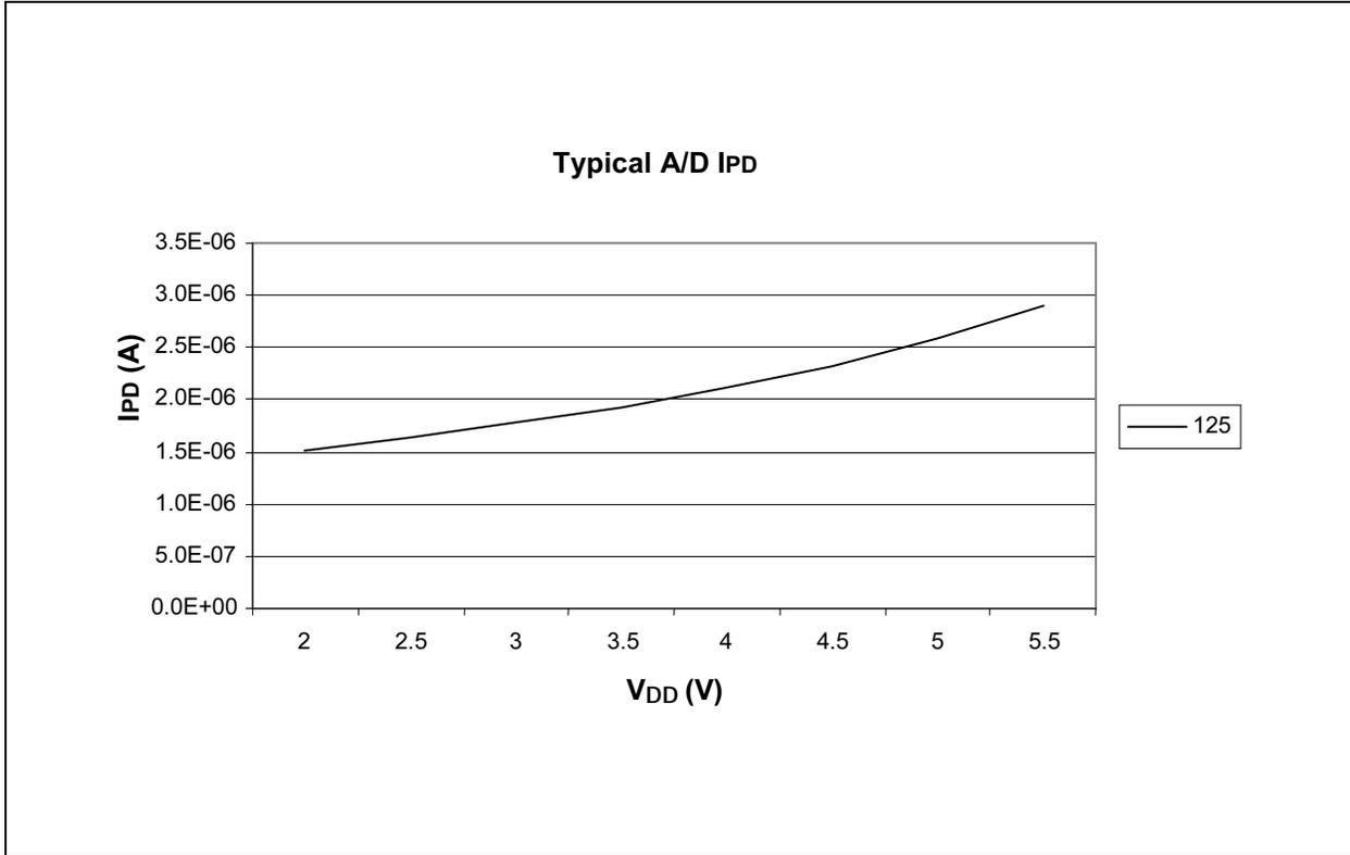
FIGURE 13-12: TYPICAL IPD WITH T1 OSC ENABLED vs. V<sub>DD</sub> OVER TEMP (-40°C TO +125°C), 32 KHZ, C1 AND C2=50 pF)
