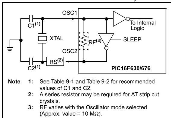
**FIGURE 9-2: EXTERNAL CLOCK INPUT OPERATION (HS, XT, EC, OR LP OSC CONFIGURATION)**
