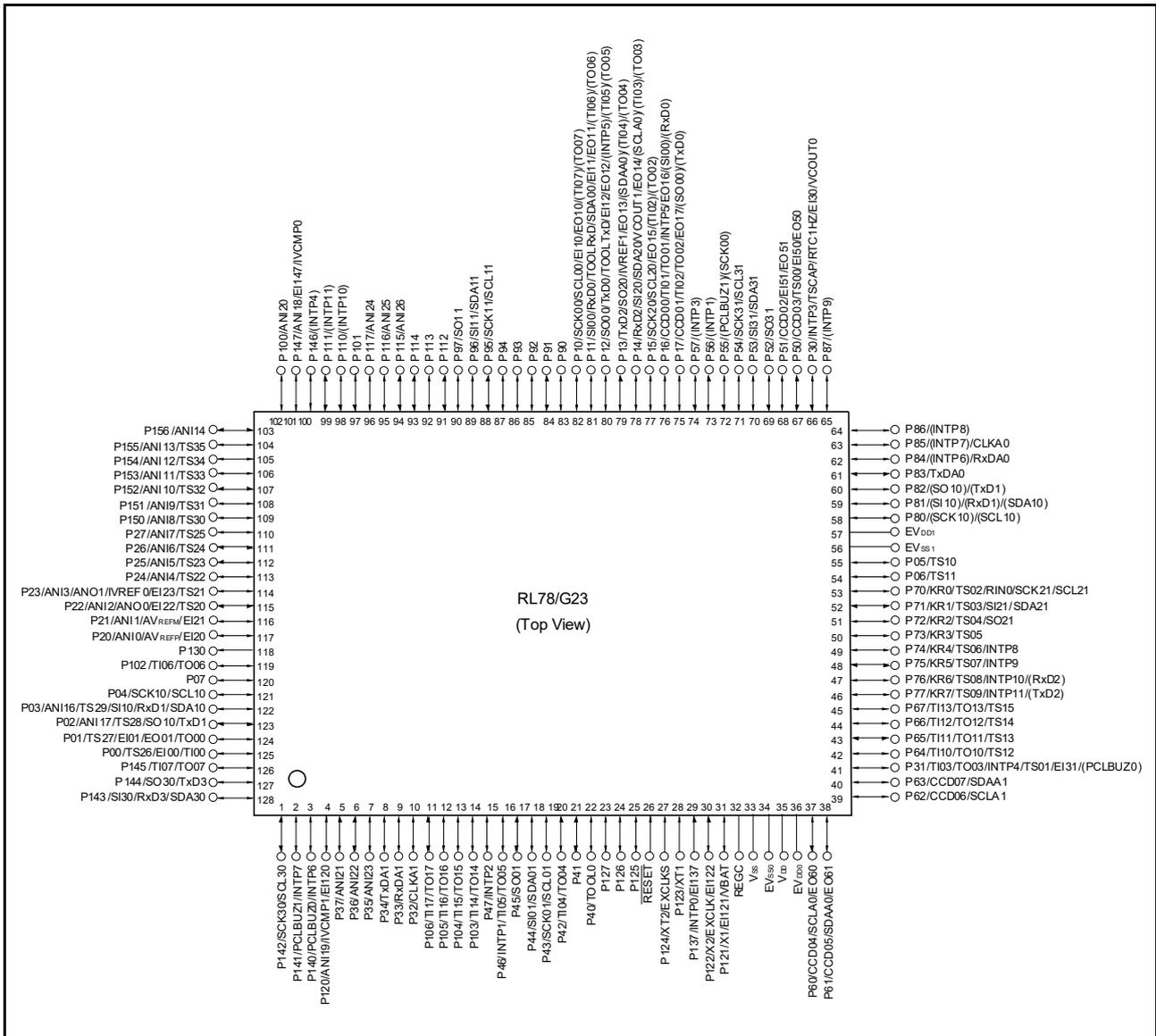
**Caution 1.** Connect the EVSS0 and EVSS1 pins to the same ground as the VSS pin.
