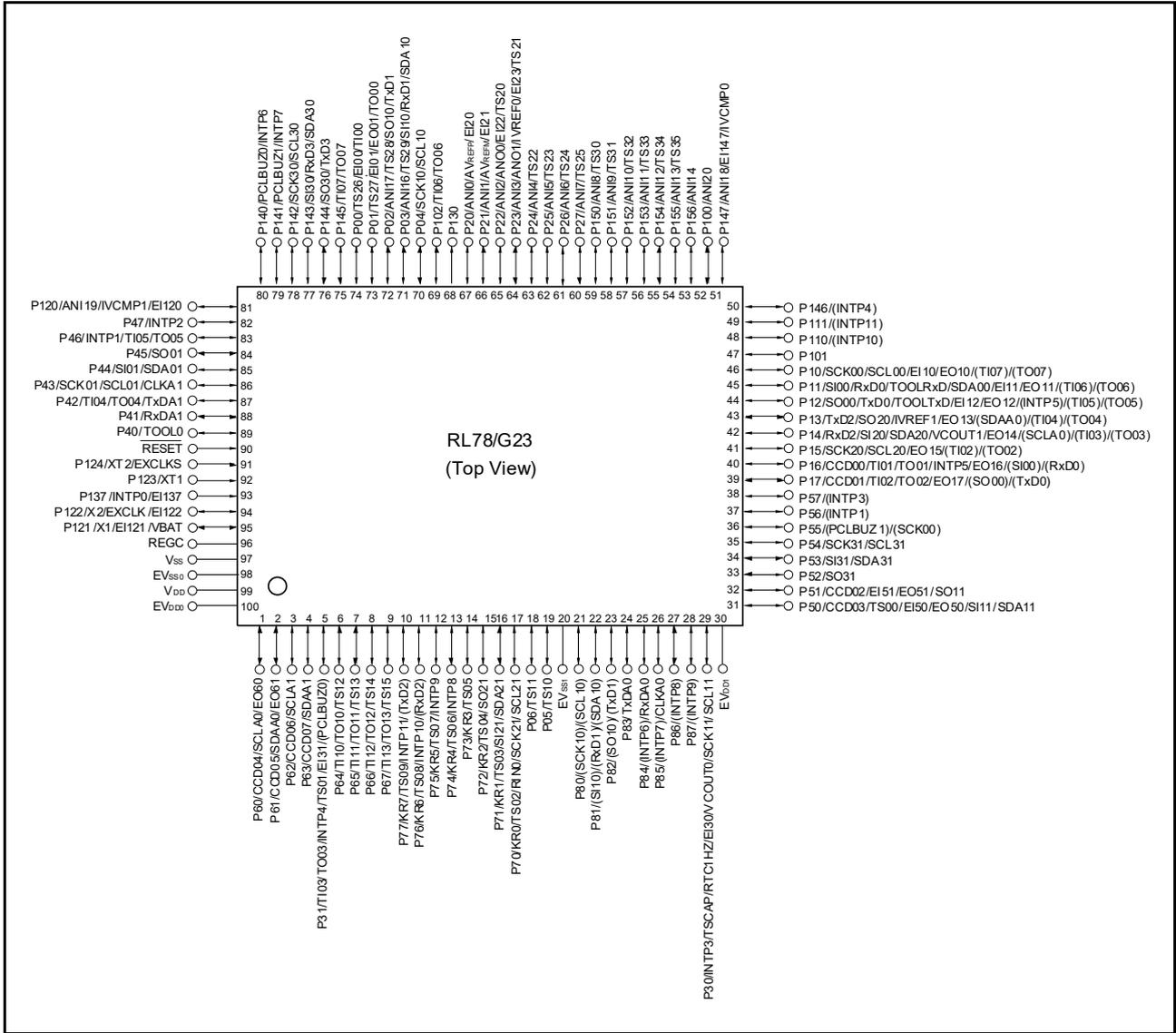
**Caution 1.** Connect the EVSS0 and EVSS1 pins to the same ground as the VSS pin.
