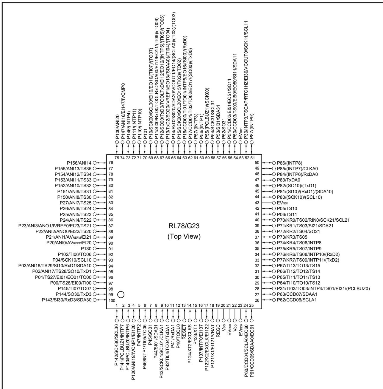
**Caution 1.** Connect the EV<sub>SS0</sub> and EV<sub>SS1</sub> pins to the same ground as the V<sub>SS</sub> pin.
