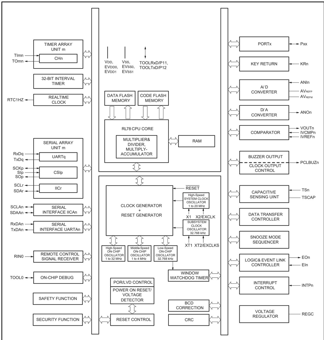
**Caution 1.** 32- to 128-pin products incorporate the remote control signal receiver.
