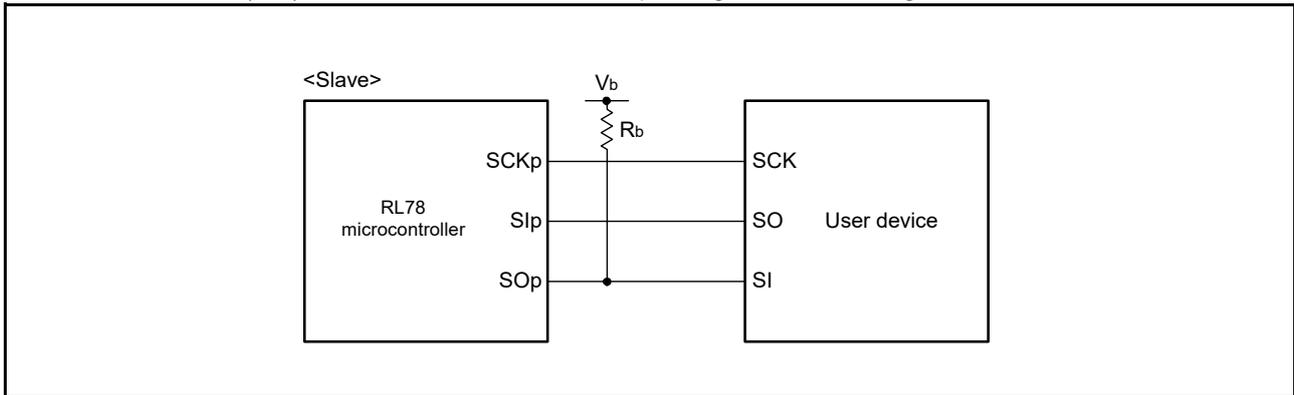
**Remark 1.** Rb[Ω]: Communication line (SO<sub>p</sub>) pull-up resistance, Cb[F]: Communication line (SO<sub>p</sub>) load capacitance, Vb[V]: Communication line voltage
