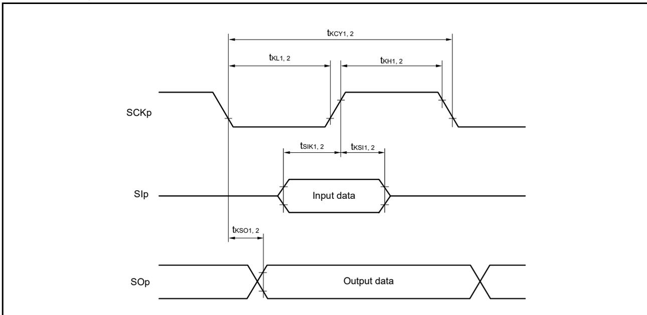
Timing of serial transfer in the SPI (CSI) communications with devices operating at same voltage levels when DAPmn = 0 and CKPmn = 1, or DAPmn = 1 and CKPmn = 0
