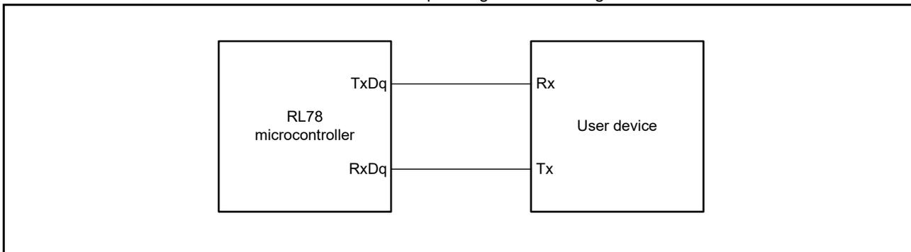
Bit width in the UART communications when interfacing devices operate at the same voltage level (reference)
