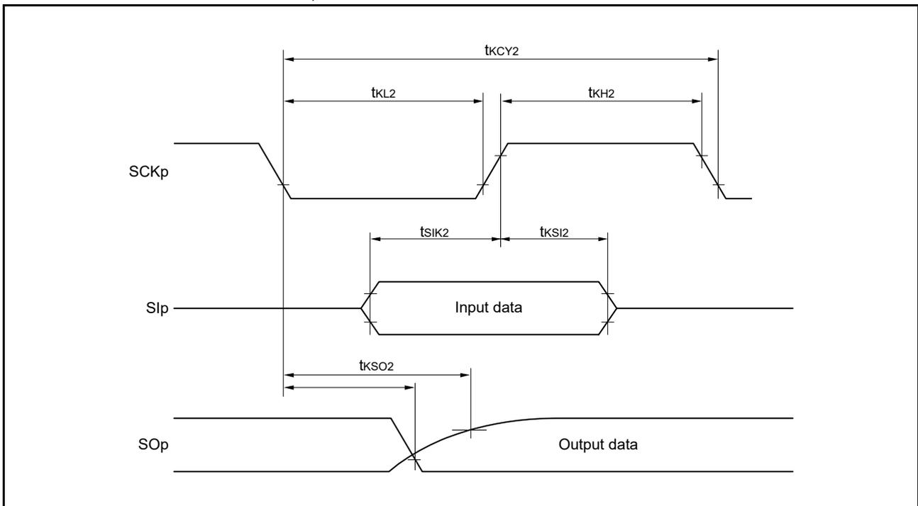
Timing of serial transfer in the SPI (CSI) communications in the slave mode with devices operating at different voltage levels when DAPmn = 0 and CKPmn = 1, or DAPmn = 1 and CKPmn = 0
