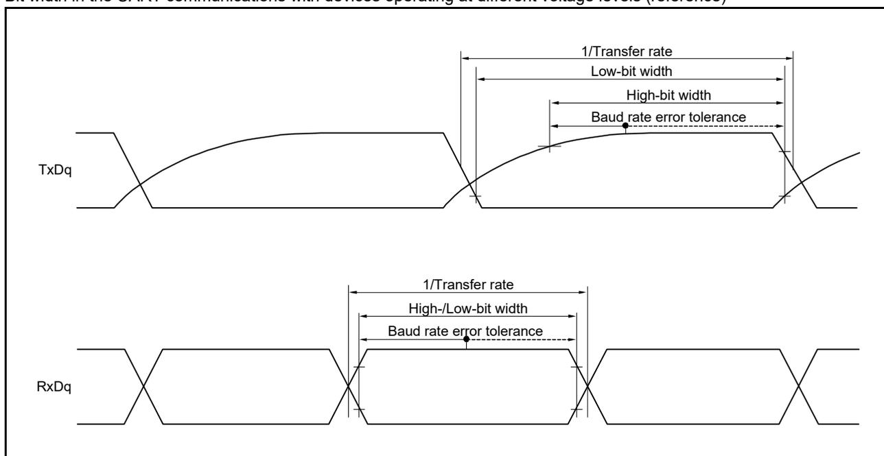
**Remark 1.**  $R_b[\Omega]$ : Communication line (TxDq) pull-up resistance,  $C_b[F]$ : Communication line (TxDq) load capacitance,  $V_b[V]$ : Communication line voltage
