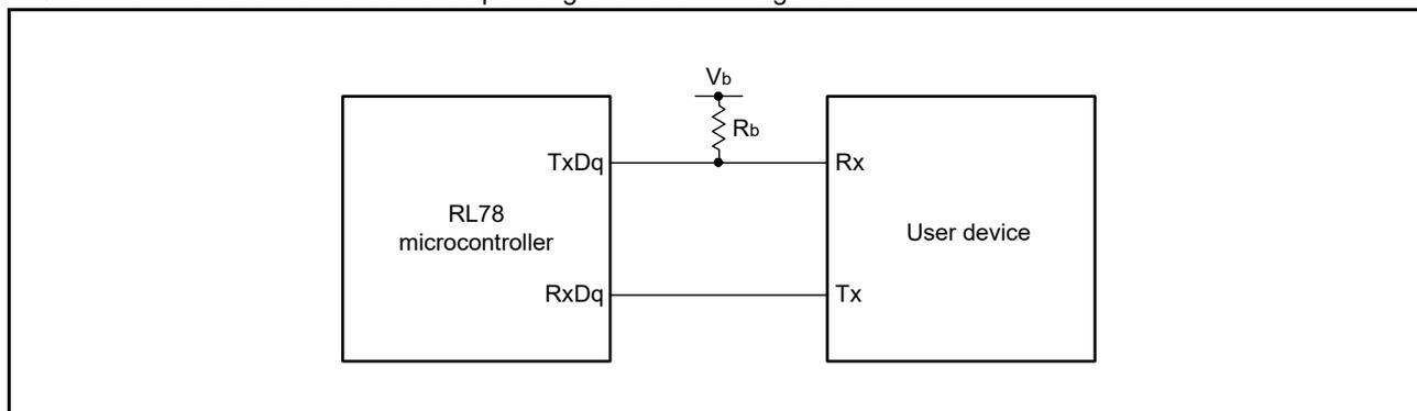
Bit width in the UART communications with devices operating at different voltage levels (reference)
