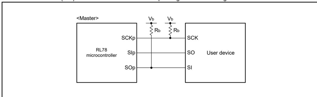
**Remark 1.**  $R_b[\Omega]$ : Communication line (SCKp, SOp) pull-up resistance,  $C_b[F]$ : Communication line (SCKp, SOp) load capacitance,  $V_b[V]$ : Communication line voltage
