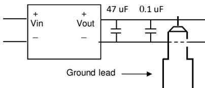
\* "Ripple and Noise" is the maximum peak-to-peak voltage value measured at the output with a 20 MHz bandwidth, at rated line voltage at full load; And with a 47µF low-ESR electrolytic capacitor in parallel with a 0.1µF ceramic capacitor across the output.
