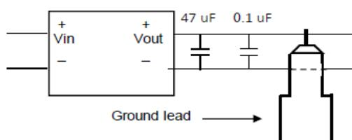
"The Ripple and Noise" is the maximum peak to peak voltage value measured at the output with a 20MHz bandwidth, At rated line voltage at full load; And with a 47uF low ESR electrolytic capacitor in parallel with a 0.1uF ceramic capacitor across the output.
