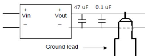
"The Ripple and Noise" is the maximum peak to peak voltage value measured at the output with a 20MHz bandwidth, At rated line voltage at full load; And with a 47uF low ESR electrolytic capacitor in parallel with a 0.1uF ceramic capacitor across the output.
