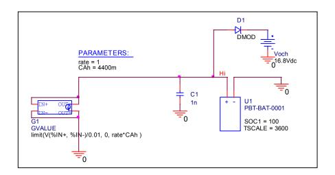
\* To discharge from 100% of battery capacity, SOC1=100
