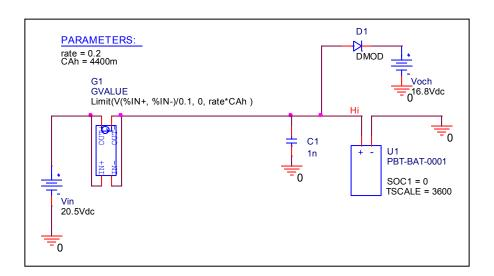
\* To charge from 0% of battery capacity, SOC1=0
