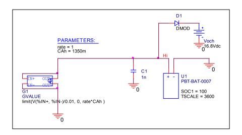
× To discharge from 100% of battery capacity, SOC1=100
