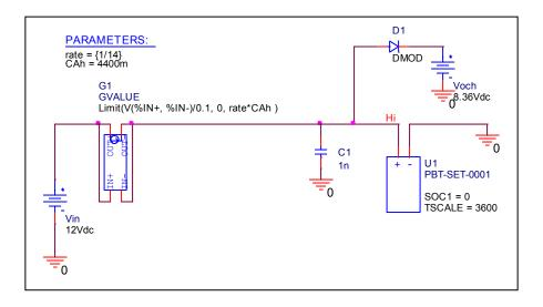
\* To charge from 0% of battery capacity, SOC1=0
